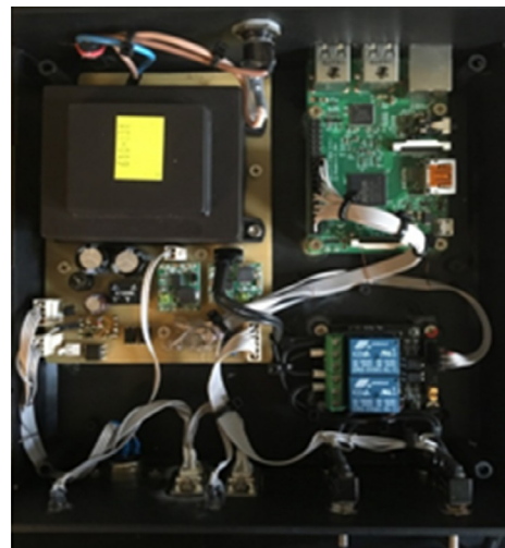
Figure 4: Block diagram (up) and her realization of smart irrigation system with all hardware components (down).
