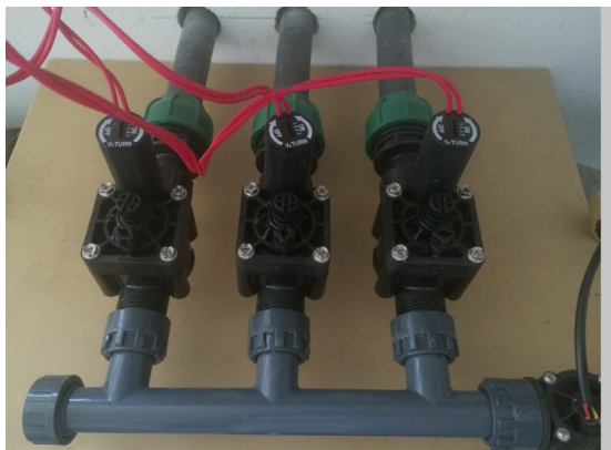
Figure 3: Connection of solenoid valves.
