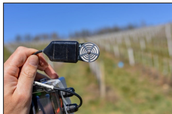
Figure 3: TEROS 21 sensor used in pilot localities.
