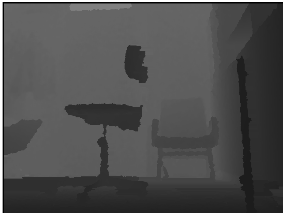
Figure 9: Depth measurement correction - error filtration algorithm (corrected frame).
