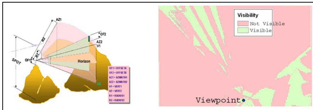
Figure 2: Schematic representation of the variables of the viewshade analysis and the result.
